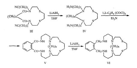
This reaction was carried out in THF at reflux over 3 h. The yield of crown ether IV was 82%. The preparation of macroheterocycle V was carried out by the cyclocondensation of macroheterocycle IV with the diacid chloride derivative of phthalic acid in benzene under high dilution conditions. The yield of macrobicycle V was 72%. The reduction of the amide groups by LiAlH<sub>4</sub> leads to cryptand VI in 80% yield.
